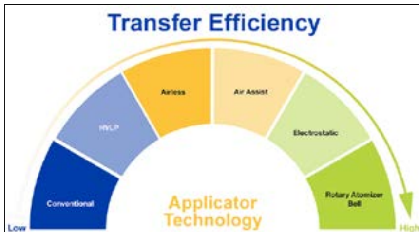
Fig 3.6.3: Transfer efficiency (graco.com)
