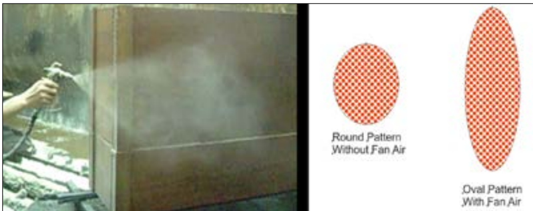
Fig 3.6.5 (iii): Conventional spray
