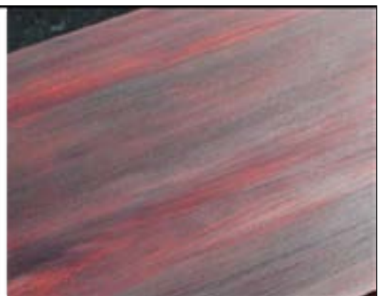
Fig 6.2.2 (xv): Dark and light stain patches
