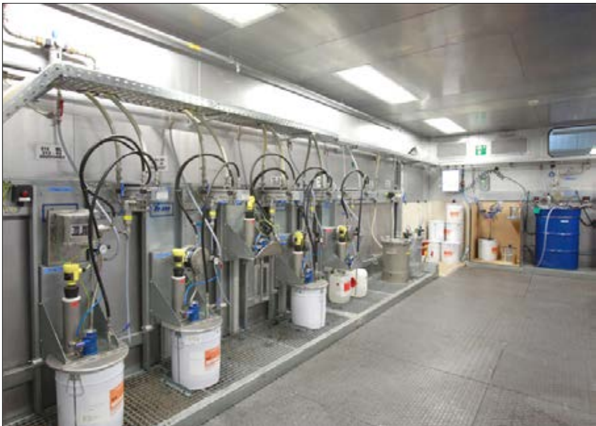
Fig 3.5: Paint circulation system (bm-systems.com)
