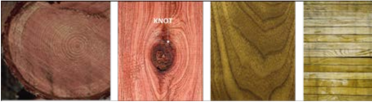
Fig 1.8.2: Rings, knots, grains and structures in the wood structure
