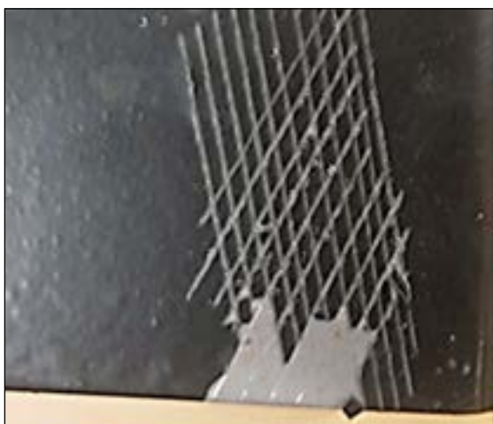
Fig 6.2.1.6 (i): Adhesion test fail
