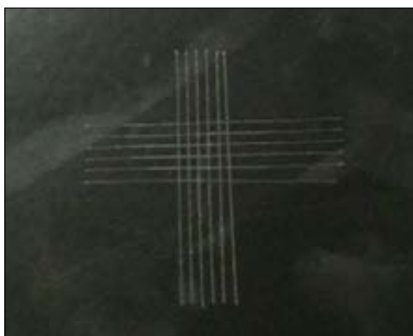
Fig 6.2.1.6 (ii): Adhesion test pass
