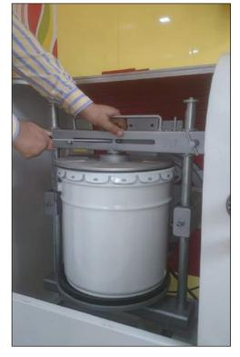
Fig 2.4 (iii): Securing the gyroshaker
