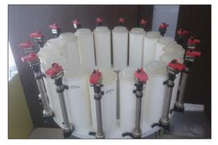
Fig 2.4 (vii): Cannisters on a carousel in a manual dispensing machine
