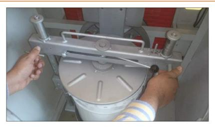
Fig 2.4 (iv): Securing the gyroshaker
