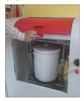
Fig 2.4 (vi): Closing the gyroshaker
