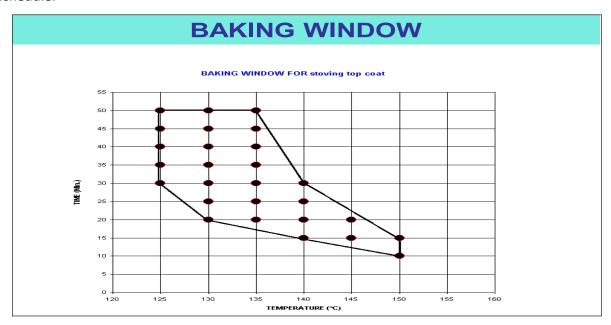
Fig 4.3.1 (ii): Baking window
