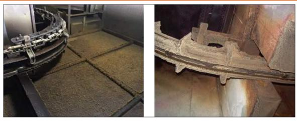
Fig 5.1.4 (ii): Dust deposited surrounding the conveyor Fig 5.1.4 (iii): Flammable condensed deposits that must becleaned
