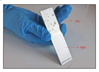
Fig 3.1.3 (i): Water break test (btglabs.com)
