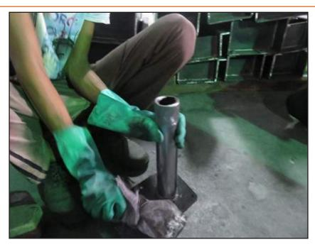
Fig 2.1 (ix): Solvent wipe before blasting
