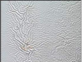
Fig 7.2.2 (vii): Mud cracking
