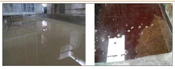
Fig 5.1.2 (i): Correct and incorrect maintenance of pretreatment baths
