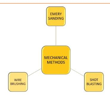
Fig 3.1.1 (ii): Mechanical pretreatment
