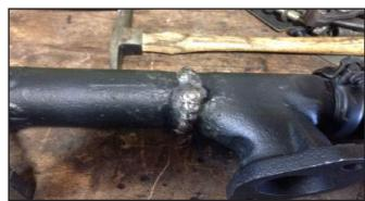
Fig 2.1 (iii): Defect in welded component
