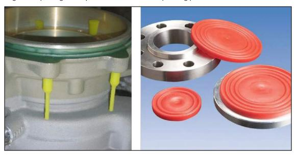
Fig 2.5 (i): Masking with plugs
