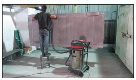
Fig 2.1 (viii): Vacuum cleaning after blasting operation
