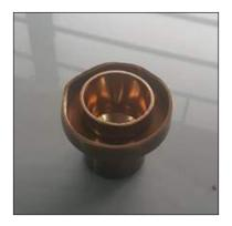
Fig 4.1 (iv): Ford cup to adjust viscosity
