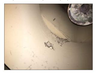
Fig 5.1.6 (v): Dust in oven burner chamber that must be cleaned
