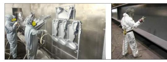
Fig 4.2.6 (i): Spray application on plastic components and metal components
