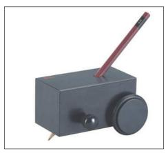
Fig 7.2.1.5: Pencil Hardness Test
