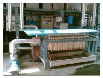
Fig 3.1.7 (ii): Filter press for online sludge removal
