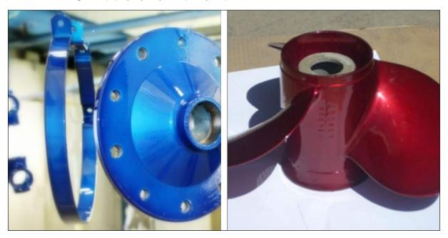
Fig 1.3.8 (iv): Polyurethane (PU) or Acrylic (Ac) applied on industrial parts
