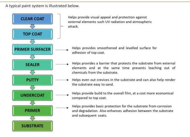
Fig 1.3.5: A typical paint system for automotive coating
