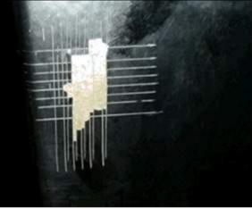
Fig 7.2.2 (xv): Poor pencil adhesion
