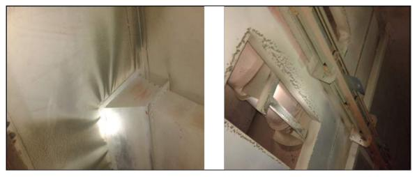
Fig 5.1.6 (ii): Inside oven dust deposits to be cleaned
