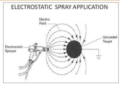
Fig 4.2.8 (iii): Electrostatic spray application
