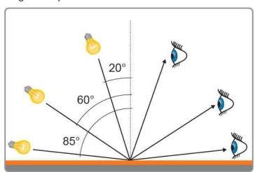
Fig 1.7: Reading gloss at different angles
