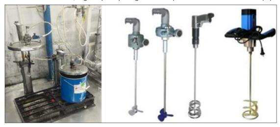
Fig 4.1 (ii): Different types of paint mixing stirrers
