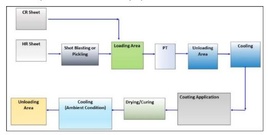
Fig 3.1: Coating process flow diagram
