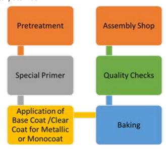
\*For plastics, special conductive primer is necessary before electrostatic application to have conductivity
