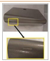
Fig 7.2.1.4: Bend test on a conical mandrel
