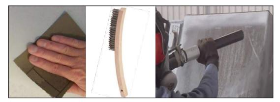
Fig 3.1.1 (iii): Mechanical pretreatment methods - emery sanding, wire brushing, blasting
