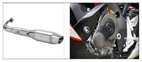
Fig 4.2.12 (i): Motorcycle silencer and engine cover
