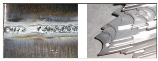
Fig 2.1 (vi): Defects that must be checked before pretreatment - Weld spatters and sharp edges.
