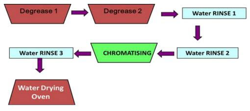
Fig 3.1.5: Schematic chromatising process chart
