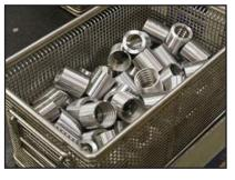
Fig 2.1 (iv): Antirust oil should provide protection during storage
