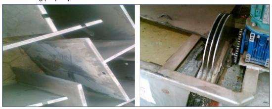
Fig 3.1.7 (i): White powder formation on phosphate layer Fig 3.1.7 (ii): Oil separators for degreasing bath
