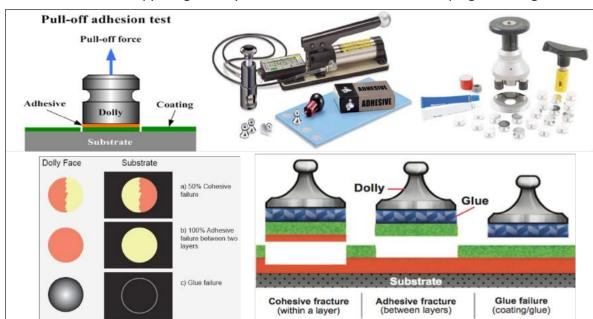
Fig 7.2.1.6 (iii): Pull-off Adhesion Test
