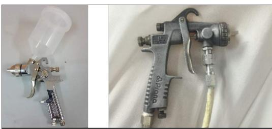
Fig4.2.4 (i): Gravity feed spray gun and suction feed spray gun
