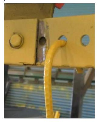
Fig 5.2.3 (i): Powder deposits on jigs will prevent proper earthing
