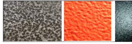
Fig 1.6 (ii): Hammer tone finish, structure finish and coarse texture
