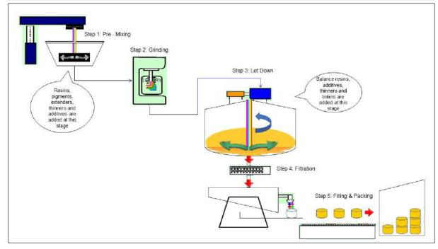
Fig 1.3.3: The main stages in the manufacturing process
