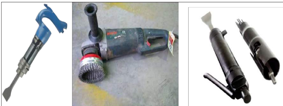
Fig 2.2.1 (vi): Rotary Wire Brush
