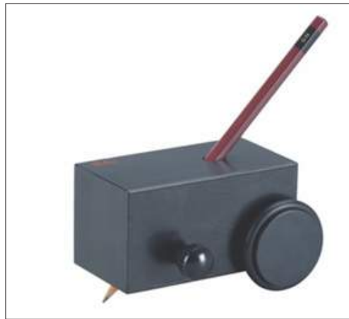
Fig 4.2.1.5: Pencil Hardness Test
