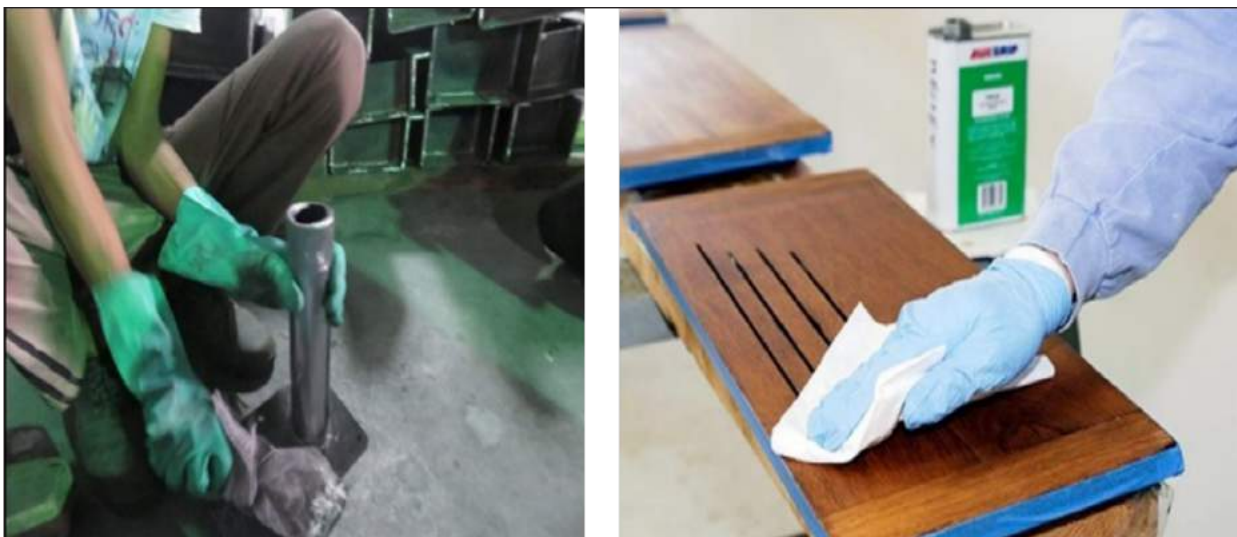
Fig 2.2.1 (ii): Solvent cleaning with a soft swab
