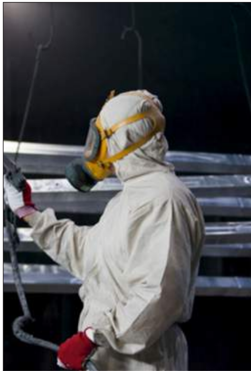
Fig 5.3 (iii): Worker with a paint mask
