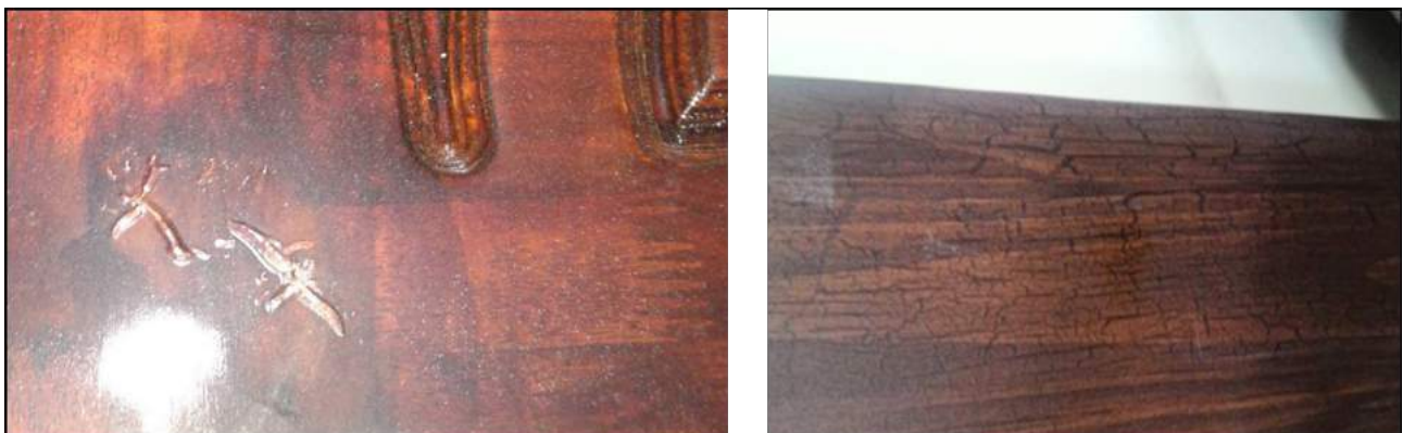
Fig 5.2.2 (vi): Wrinkling / lifting
