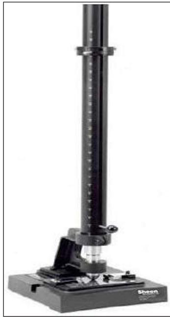
Fig 5.2.1.7 (i): Impact Tester Fig 5.2.1.7 (ii): Impact Test
