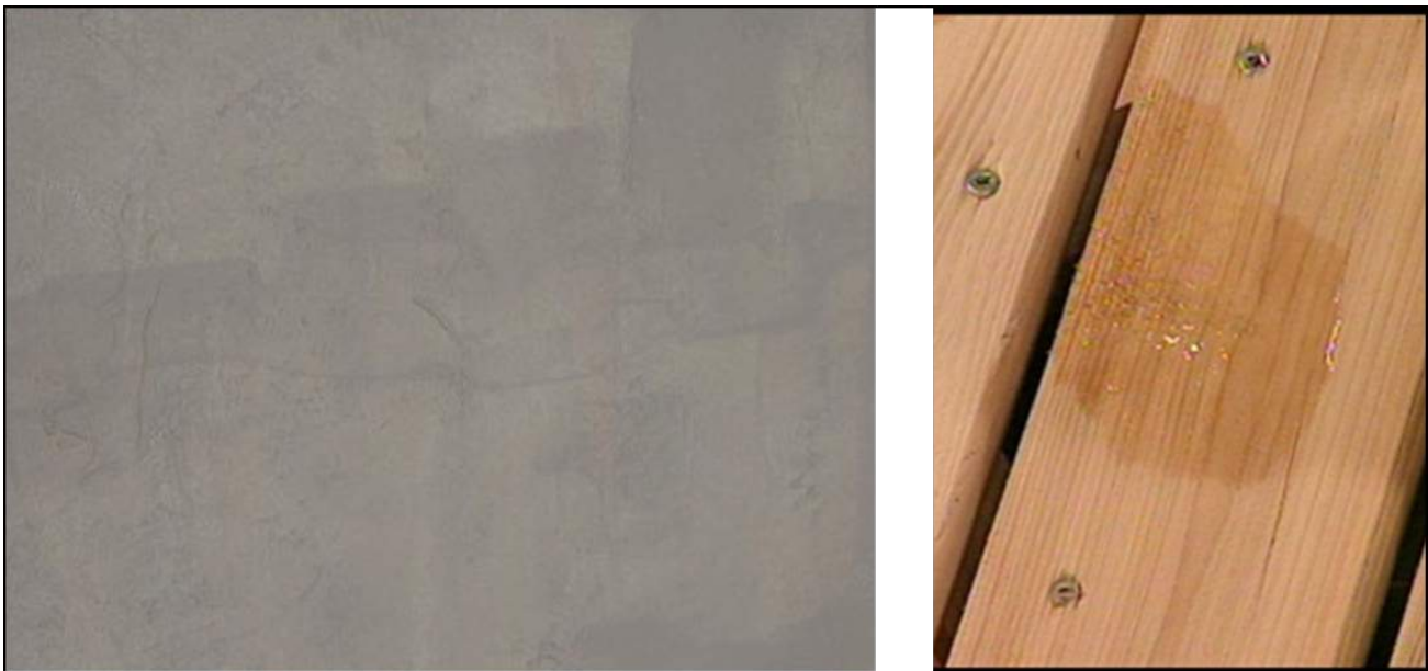
Fig 5.2.2 (v): Uneven film thickness
