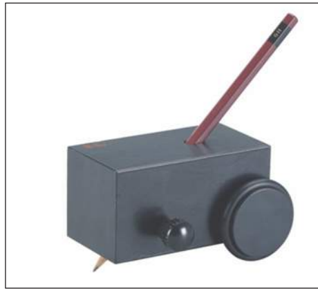
Fig 5.2.1.5: Pencil Hardness Test
