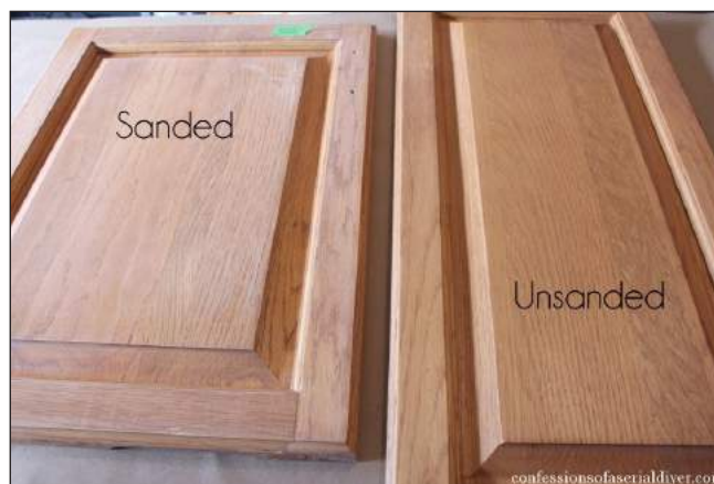
Fig 3.2.1: Visual difference between sanded and un-sanded components (confessionsofserialdiyer.com)
