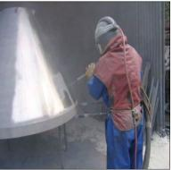
Fig 3.1 (vii) Manual abrasive blasting
