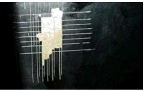
Fig 7.8 (xv) Poor pencil adhesion
