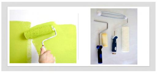
Fig 3.3 (ii) Roller application and Anatomy of a Roller
