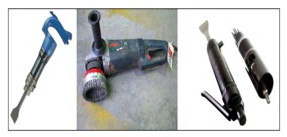
Fig 3.1 (vi) Rotary Wire Brush
