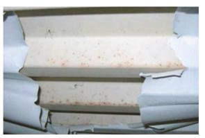
Fig 7.8 (x) Inter-coat delamination
