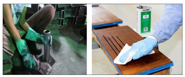
Fig 3.1 (ii) Solvent cleaning with a soft swab
