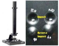
Fig 7.7 (i) Impact Tester Fig 7.7 (ii) Impact Test
