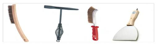
Fig 3.1 (v) Tools used in hand cleaning
