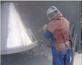
Fig 2.2.1 (x): Manual abrasive blasting
