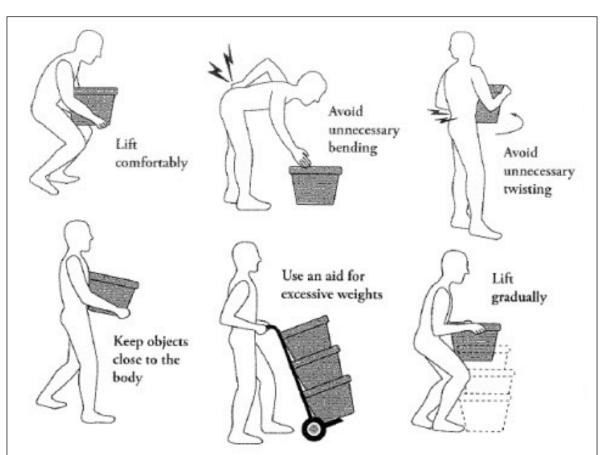
Fig 5.5.1 (i): Correct lifting techniques (worldartsme.com)
