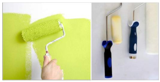
Fig 2.4 (ii): Roller application and anatomy of a roller
