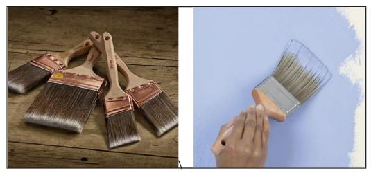
Fig 2.4 (i): Variety of paint brushes and paint application with brush (homedepot.com, diynetwork.com)
