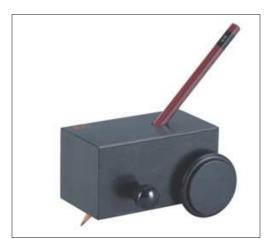
Fig 4.2.1.5: Pencil Hardness Test
