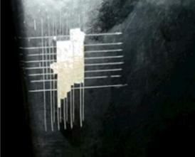
Fig 4.2.2 (xv): Poor pencil adhesion
