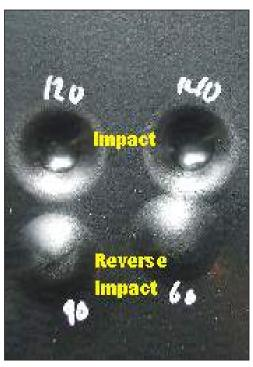
Fig 4.2.1.7 (ii): Impact Test
