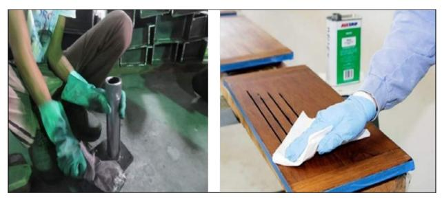
Fig 2.2.1 (ii): Solvent cleaning with a soft swab
